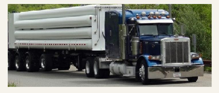
When it comes challenging terrain, long distances or the lack of large consumption centers, the installation of conventional pipelines becomes unfeasible. Under these conditions, the Virtual Pipelines connect consumers to the gas network last miles.
